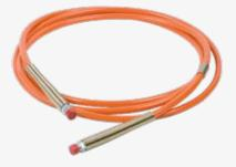
When working with high pressure hydraulics 700 Bar / 10.000 psi safety comes first. All Holmatro hoses are suitable for 700Bar working pressure. Our hoses are designed on a 4:1 safety ratio, resulting in a 10 year lifespan. All hoses are individually tested during the production proces.
