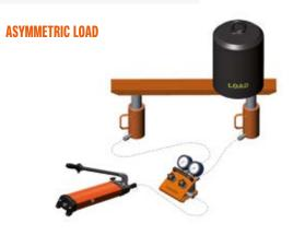
Recommended total cylinder capacity = 2 x load
