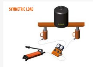
Recommended total cylinder capacity = 1.5 x load
