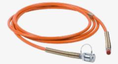
When working with high pressure hydraulics 700 Bar / 10.000 psi safety comes first. All Holmatro hoses are suitable for 700Bar working pressure. Our hoses are designed on a 4:1 safety ratio, resulting in a 10 year lifespan. All hoses are individually tested during the production proces.
