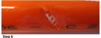
Replace the Core hose when damage is such that the one braided layer of high tensile synthetic fibre is clearly visible.
