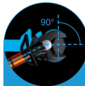
Inclined cutter blades keep the ideal 90° angle towards the construction, required for effective cutting. Any other position will reduce cutting performance.
