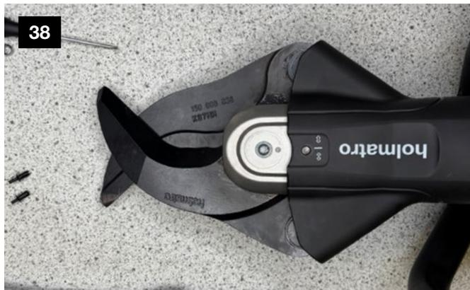
Unfold the protection sleeve
