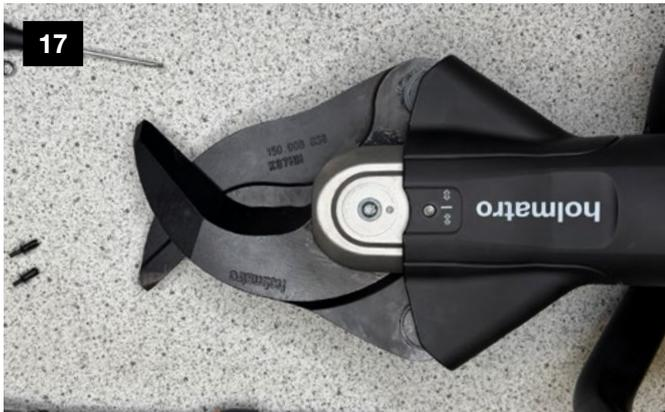
Unfold the protection sleeve
