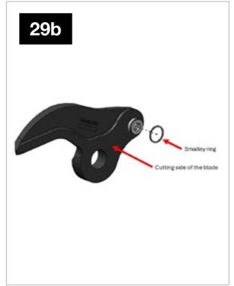
Mount the hinge pins with the smalley ring on the cutting side of the blade
