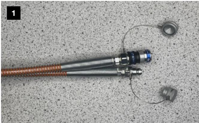
Only for HMC: Check hoses & couplers for leaks, dirt, and damage
